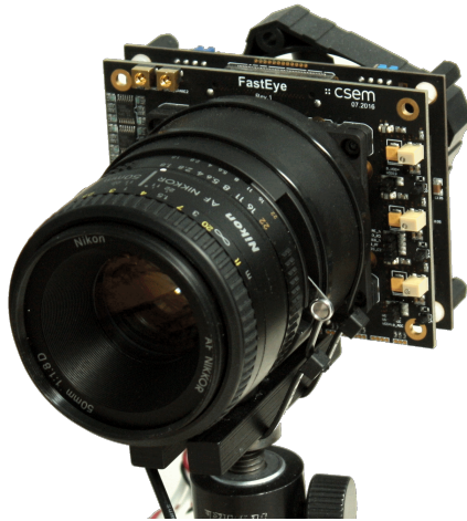
Figure 3.3: Image of the presented camera system with a mounted objective.
