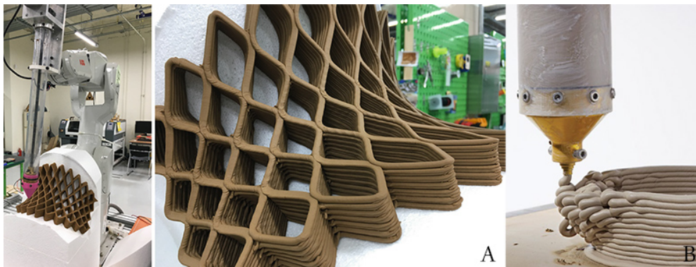
FIGURE 2.3: Clay Fabrication and Failure: A. 3D printed clay object on a customized doubly-curved base (Ko et al. 2019); B. 3D printing clay collapses during the fabrication. (Rael and Fratello 2017).
