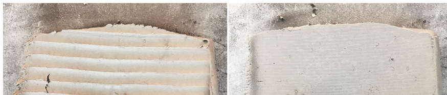
FIGURE 5.8: Surface quality differences due to a non-flat profile loop. The local stripe effect caused by the leftovers between toolpaths is homogeneous with the tools. For a loop tool with selected shape, the user can adjust this parameter to obtain a desired final appearance.
