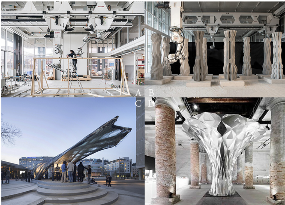
FIGURE 1.2: Various researches and applications of digital fabrication in the architecture field: A. Spatial Timber Assemblies , timber frames assembled by robot arms (Gramazio Kohler Research, ETH Zurich); B. Concrete 3D Printed Columns (Digital Building Technologies, ETH Zurich) ; C. 2017 Institute for Computational Design and Construction (ICD) Research Pavilion (ICD, ITKE University of Stuttgart) ; D. ARUM , robotically folded steel sheet structure (RoboFold & Zaha Hadid Architects).
