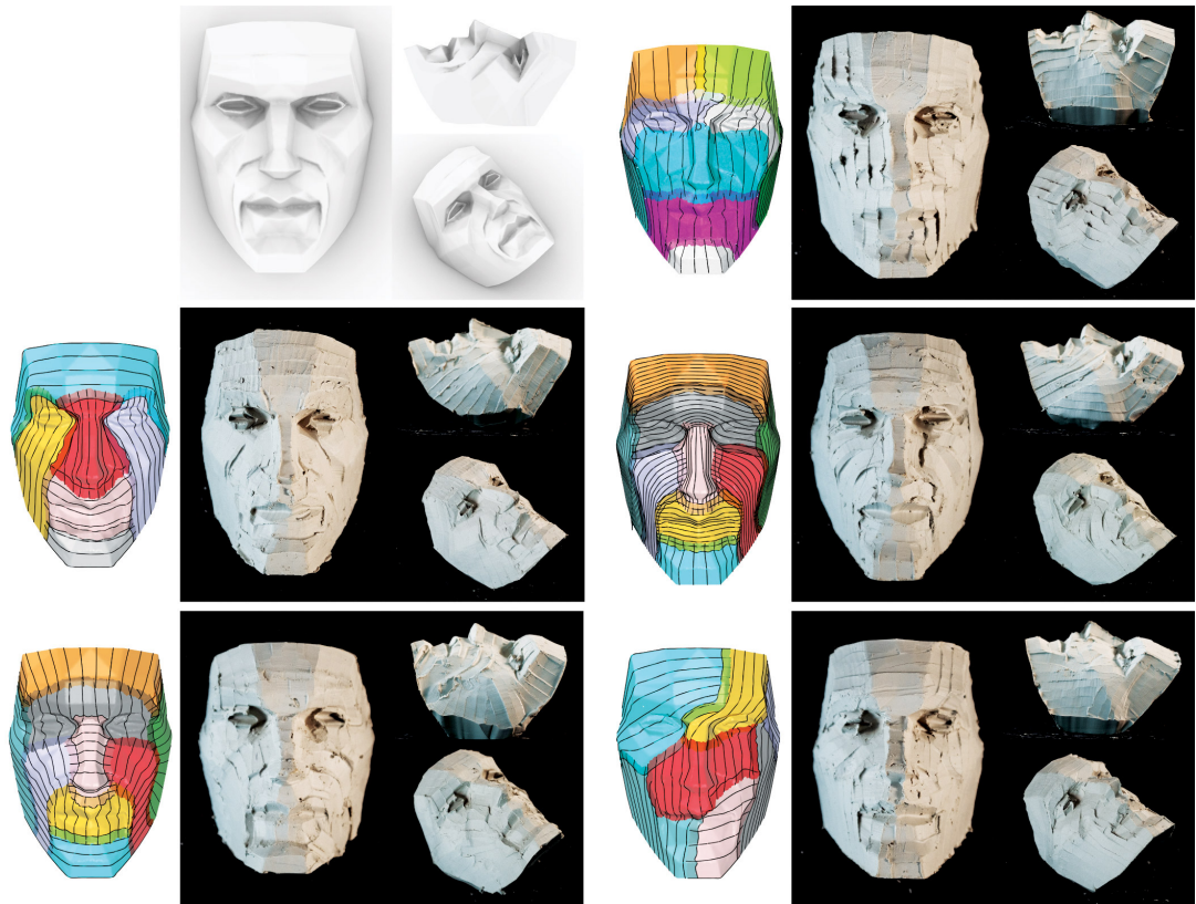
FIGURE 5.20: Sculpting results of the face model. Top-left: the input geometry; Rest: initialized toolpaths and the results with different styles by executing robot trajectories generated from RobotSculptor .
