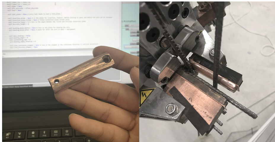
FIGURE 4.10: The modified bronze metal part (left) and a work-in-progress clamp with one side metal part replaced (right).
