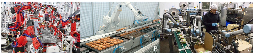
FIGURE 1.1: Robot arms in industrialized environment. A. Tesla assembly line; B. Food assembly line; C. Human-Robot collaborative assembly line.
