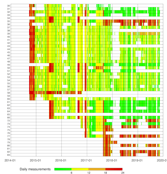
Figure 6. Availability of TPS2 (Leica TM50) measurements over the monitoring period. The target ID is shown in the y -axis (for the location of targets see Figure 1), while the colormap shows the amount of daily measurement cycles performed.
