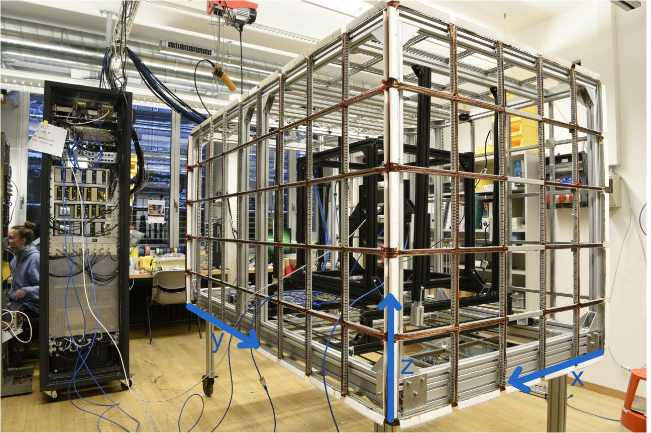
Figure 4.1: Photograph of the AMS prototype in the ETH laboratory at Höggerberg. The side facing the window front is open in order to enable to place a mu-metal cube inside. The origin is in the bottom left corner closest to the windows.
