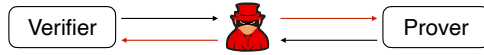
Figure 2.3: In Mafia Fraud, an external attacker reduces the distance measured between two mutually trusted parties.
