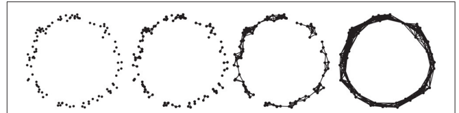
FIGURE 2 | Different stages of a Vietoris–Rips filtration for a simple “circle” point cloud. From left to right, connectivity of the underlying simplicial complex increases as \epsilon increases.
