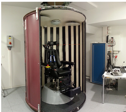
(a) Optokinetic drum used for the vection test. Subjects sit inside the drum with their head fixed and fixate on a point on the rotating wall
