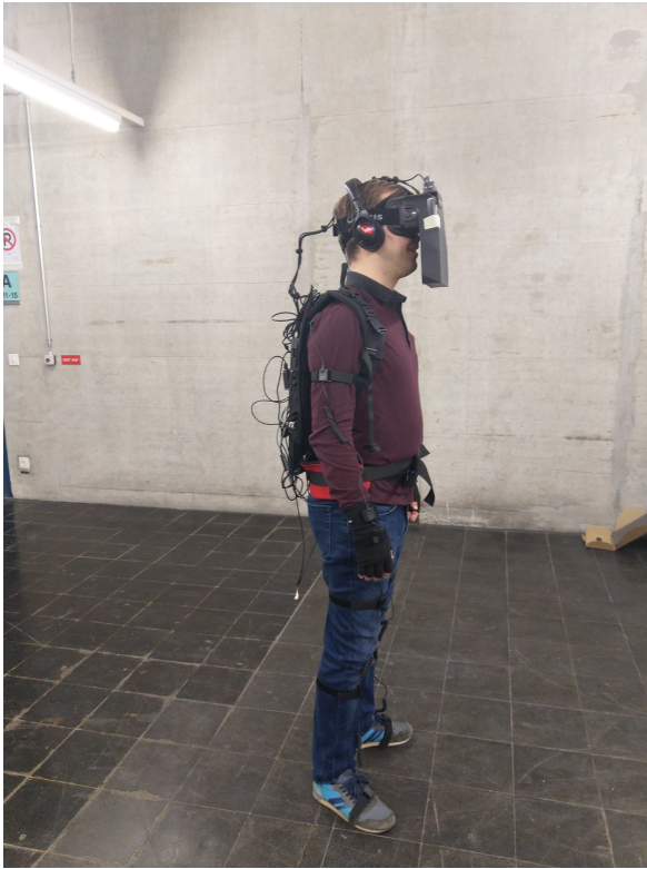
(a) Experiment set-up with the Intersense IS-1200 tracking 6-DOF head position, and the Noitom motion suit tracking body movement
