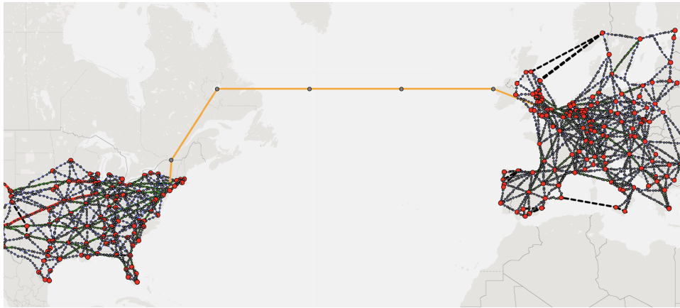
Figure 6.6: An envisioned trans-Atlantic low-latency hybrid network consisting of LEO satellites, terrestrial radio, and fiber.
