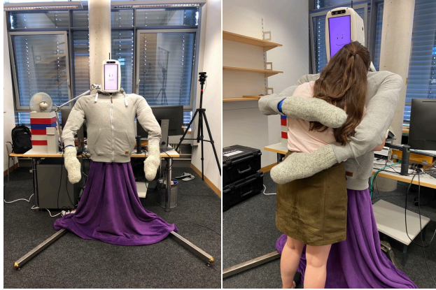
FIGURE 6.2: Views of HuggieBot 2.0 (Block, Christen, et al., 2021) ready for a hug and hugging a user. This custom human-sized hugging robot has two padded arms, an inflated torso, and a face screen mounded to a rigid frame. A camera above the screen visually senses the user at the start of the interaction, and torque sensors on the shoulder flexion and elbow flexion joints are used to embrace the user with a comfortable pressure. A microphone and pressure sensor in the back chamber of the torso are used to detect user contact and detect and classify gestures. The user ends the hug by releasing the robot’s torso and/or leaning back against the arms.
