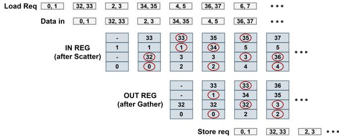
Fig. 3. Buffer-less FFT HWPE pipeline. The example shows the beginning of a 64-point  $C64$  FFT first stage. One  $C64$  sample occupies one 64-bit register. In case of lower-precision FFTs, samples are packed inside 64-bit registers.
