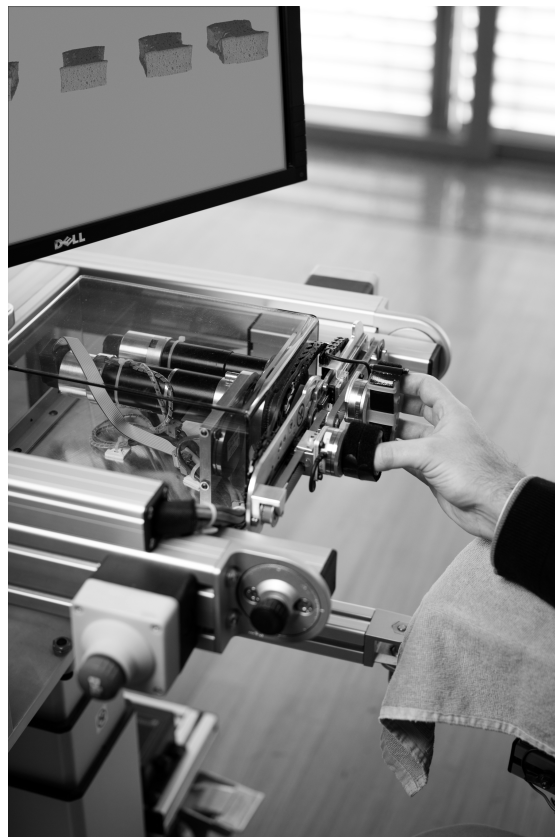
Figure 2.1: A subject with stroke using the ReHapticKnob. The ReHapticKnob is a haptic device used to train hand opening-closing and forearm pronosupination. The device integrates a set of 7 therapy exercises reproducing typical neurocognitive exercises [Metzger et al., 2014b]. In the present exercise, the compliance of different virtual sponges rendered by the device has to be memorized and identified by relying on hand somatosensory inputs during active interaction with the device.
