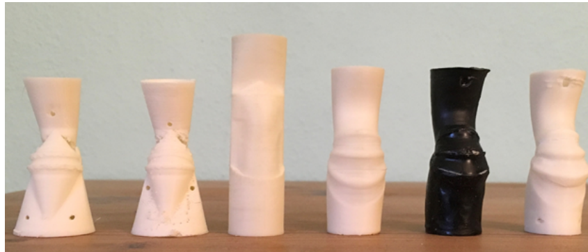
Figure 4.8: Evolution of actuator design. Shown are a selection of the iterations made to achieve the final design. The first two designs were drawn with Solidworks. Bowden extrusion led to printing errors and the pivot point constantly ripped. The third design was a complete restart with new drawings using Fusion 360 and direct extrusion. Very thin membranes (0.4 mm) could be achieved. The next design had better working pivot point, but the sliding and dimensions of the hoops were not right yet and resulted in membrane ripping. The black print is the final design but sealed with PlastiDip. On the very right, the final design with a thin latex layer on the inside to seal any printing irregularities.
