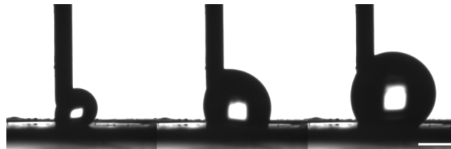
Figure 3.20: Contact angle measurement of water on artificial microstructured membrane. Water droplet on microstructured parylene coated artificial membrane ( 5\ \mu\text{m} ). Preliminary analysis showed contact angles of 100 - 115^\circ . Scale bar: 0.5\ \text{mm} .
