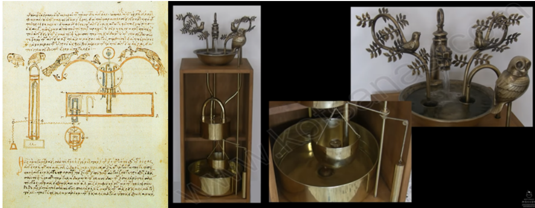
Figure 4.1: Ancient Greek hydraulic automata. Left: Technical Drawing of chirping bird automata from the Pneumatica book by Heron of Alexandria. Photography taken from Wikimedia Commons. Right: Rebuild bird automata in museum of ancient greek technology 1 by Kostas Kotsanas. Screenshot from Youtube Video 2
