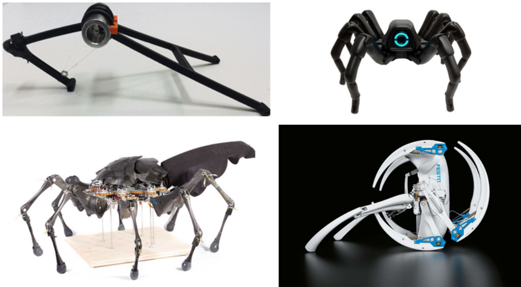
Figure 4.2: Level 1 Spider Inspiration. Top left: Jumping performance depending on the leg angle [36]. Top right: Omnidirectional, realistic spider robot (Robugtix, T8X) 4 using servomotor joints. Bottom left: ARAC ETH focus project 5,6 using tendon driven legs. Bottom right: Festo BionicWheelBot 3 uses spring-motor actuators to allow rolling and walking motion inspired by the desert spider Cebrennus rechenbergi .
