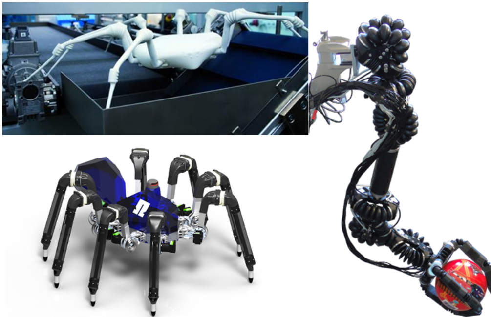
Figure 4.4: Level 3 Spider Inspiration. Top left: 3D printed Arachno-Bot 8 by Fraunhofer using pneumatic bellows for joint actuation [20]. Bottom Left: OHM-Krabbler Project 9,10 at TH Nürnberg mainly based on work by Landkammer [61] using TPU based flexible pneumatic bellows for extension and pneumatic muscles to flex the joint. Right: Robotic Arm using pneumatic bellow [42].
