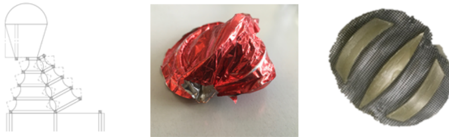
Figure 4.6: 2D to 3D membrane fabrication. Left: Cutting pattern for membrane with pockets to fill in stiffer elements. Middle: BoPET foil attached around stiff rings. Right: 3D printed PVA (polyvinyl alcohol) on fly net and subsequently cast in latex.
