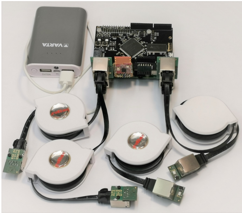
Figure 4.2: WHISPER-M4 module for COCOHA system with attached custom digital I 2 S microphones powered from a USB powerbank.
