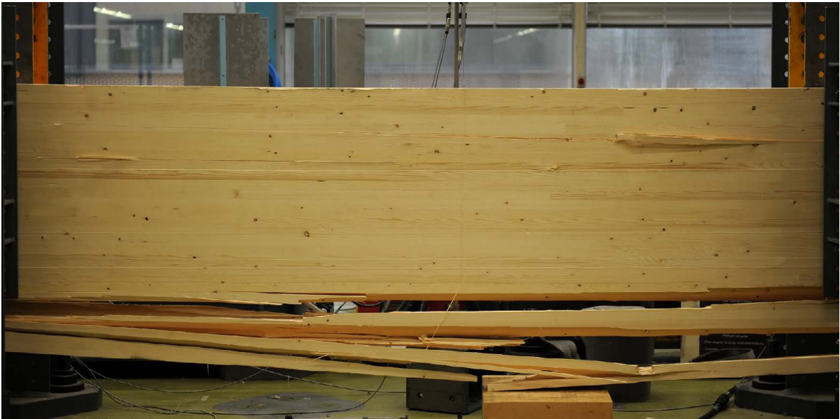
Fig. 44: Illustration of GL32h-19m-1 after ultimate failure (area between central buckling stabilisers).
