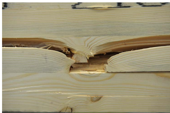
(f) 3rd lowest lamella ( l \approx 5.4 m)
