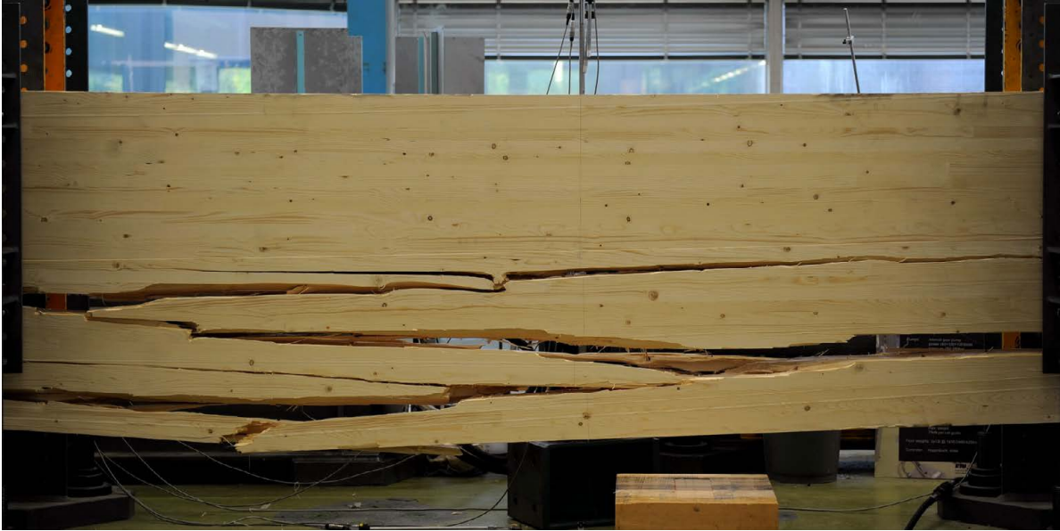
Fig. 18: Illustration of beam GL24h-19m-1 after testing (area between central buckling stabilisers)
