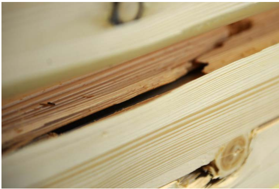
(f) 3rd lowest lamella ( l \approx 6.4 m), back side
