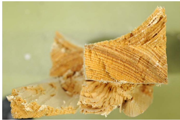
(f) failed section ( l \approx 5.0 m), back side
