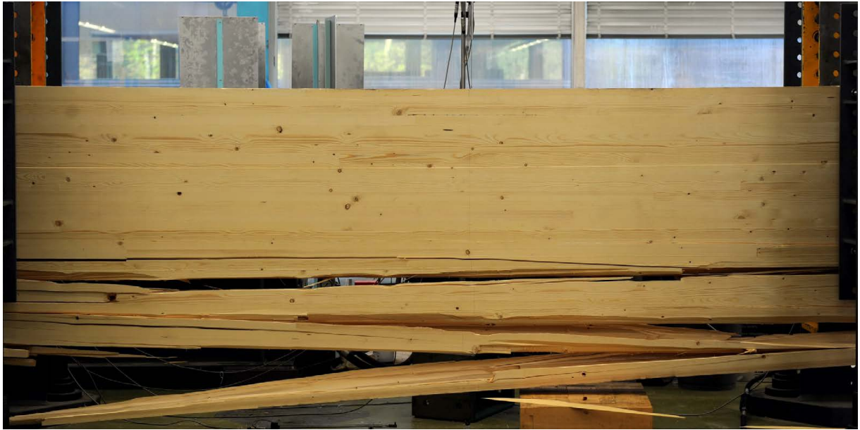
Fig. 49: Illustration of beam GL32h-19m-2 after testing (area between central buckling stabilisers).
