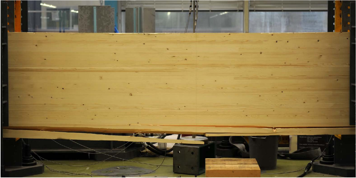
Fig. 43: Illustration of GL32h-19m-1 after first rupture (area between central buckling stabilisers).
