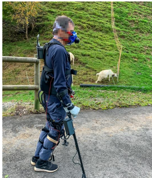
Figure 1. Photograph of the participant at the site of the outside walking experiments. The participant is wearing the Myosuit, a lightweight, cable-driven robot, and a mobile respirometer as well as forearm crutches.
