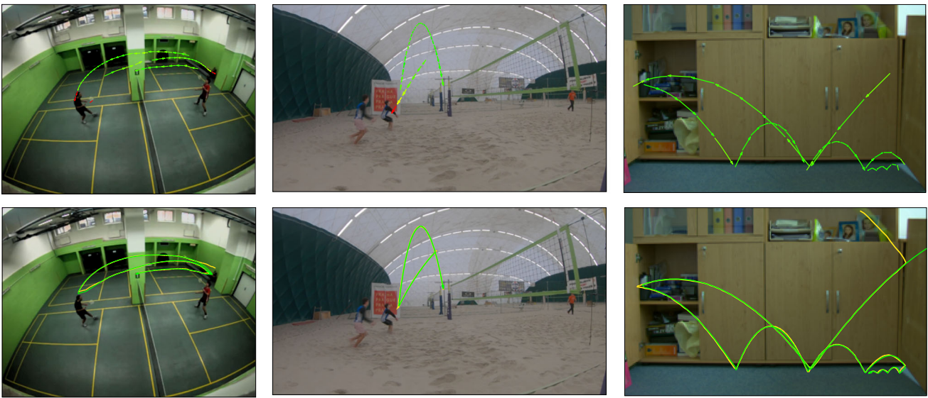
Fig. 11 Trajectory recovery for sequences selected from the TbD dataset. Top row: trajectories estimated by the causal TbD overlaid on the first frame. TIoU (14) with ground truth trajectories from a high-speed camera is color coded by scale in Fig. 10. Bottom row:
