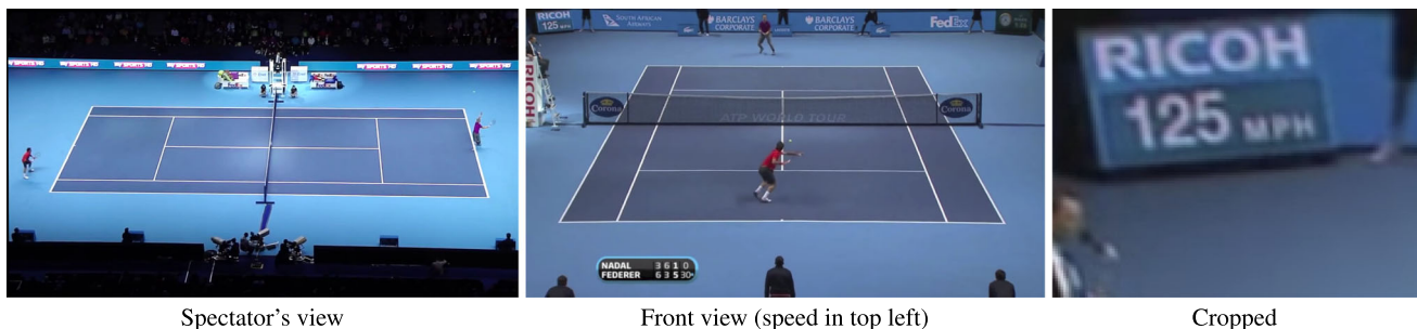
Fig. 19 Radar gun measurements. Speed was automatically estimated by the TbD-NC method from the video on the left. Ground truth acquisition from YouTube video is shown in the middle and the right images. Table 6 compares estimates to the ground truth
