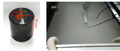
Figure 6 Photograph of simplified shape sample of the simulated fuel debris and the experimental environment under mist condition
