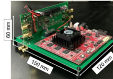
Figure 12 Developed ultrasonic measurement device (UVP-TIT SKP3)
