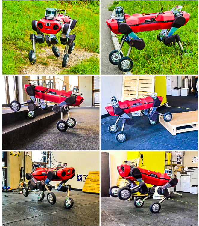
Fig. 1. With our novel whole-body MPC, the robot ANYmal [17], equipped with actuated wheels, explores indoor and outdoor environments in a fast and versatile way (video available at https://youtu.be/_rPvKlvyw2w ). First row: Locomotion in high grass and over steep hills of up to 2 m/s, while gait sequences are automatically discovered. Second row: Blindly stepping over a 0.20 m high step (32% of leg length) and stairs with a 0.175 m high step (28% of leg length). Third row: Pacing gait and 0.28 m high jump with front legs.
