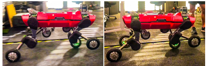
Fig. 6. High accelerations using the whole-body MPC approach. The robot executes a fast change of direction between 2 and -2 m/s, which forces the optimization problem to find complex motions that can not be captured by the LIP, as shown in Fig. 5.
