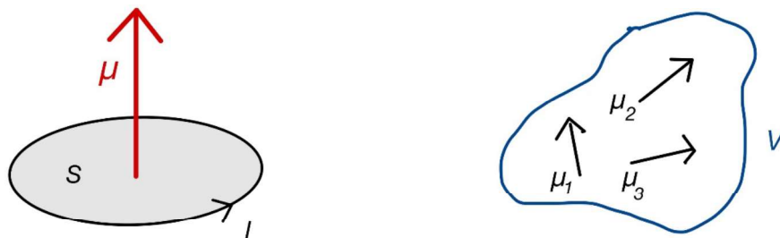
Fig. 2.1 a) Magnetic moment of electric current loop, and b) graphic representation of volume V containing magnetic moments.
