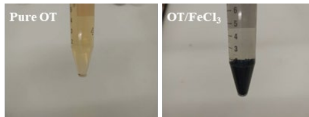
Fig. 2. Pure oak tannin solution alone (left) and with iron chloride (right). Precipitate with a dark-blue color can be seen when the tannin solution was encountered with free iron ions.
