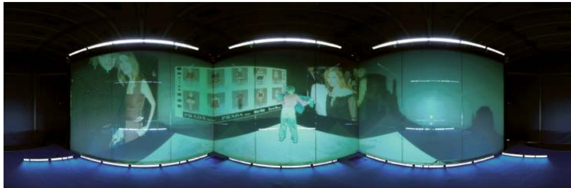
Figure 4.18: Unfolded panoramic picture of the CAVE™-like portal at ETH Center showing the three projection screens in transparent mode located in the server space of the ETH Zurich.
