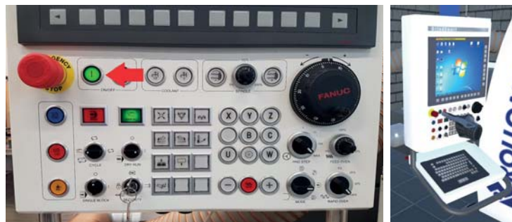
Figure 7 Real main button for the machine control and the virtual twin (see online version for colours)
