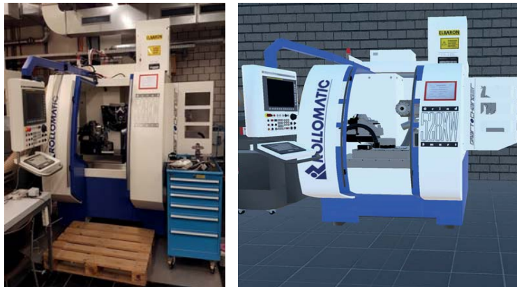
Figure 2 Real MT and the virtual twin (see online version for colours)
