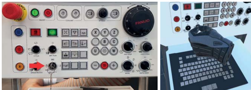
Figure 11 Locking the doors on the real control panel and the virtual twin (see online version for colours)
