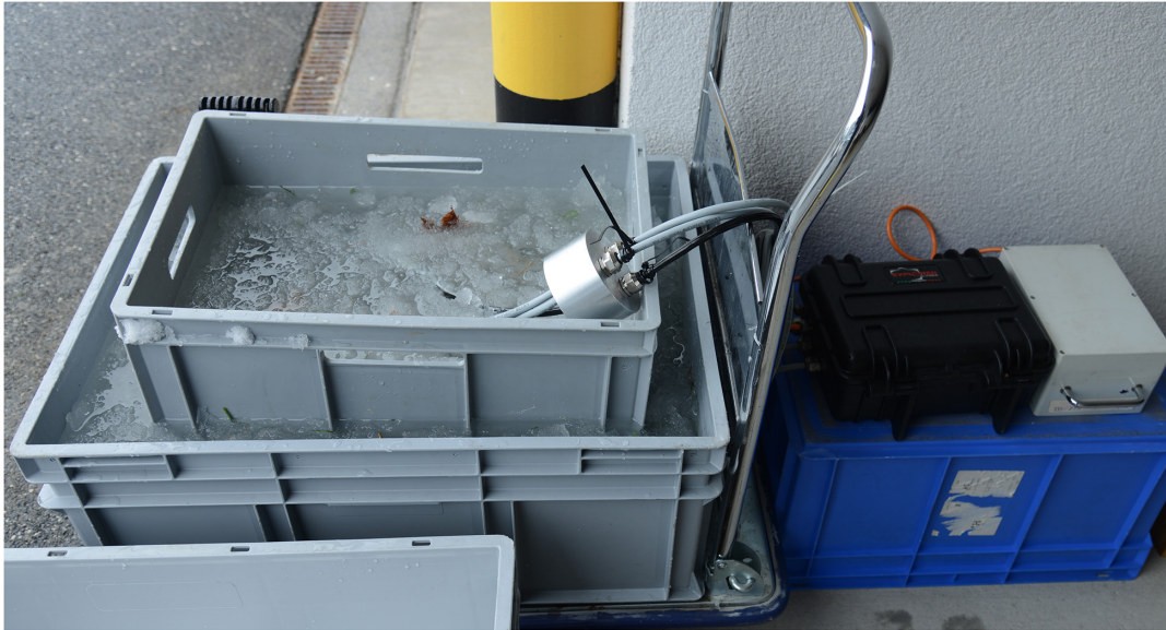
FIGURE 7 | A 0°C crushed ice-water bath for calibration of temperature sensors. The use of a double bath minimizes external temperature influences. The ice-water mixture must be stirred constantly during calibration and the temperature controlled by a high-precision reference thermometer. Photo: M. Phillips.
