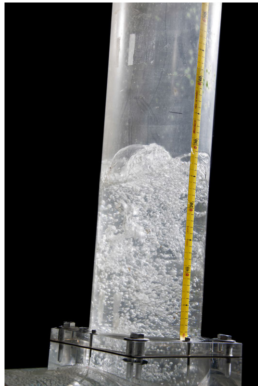
(b) De-aeration at rising pipe #2
