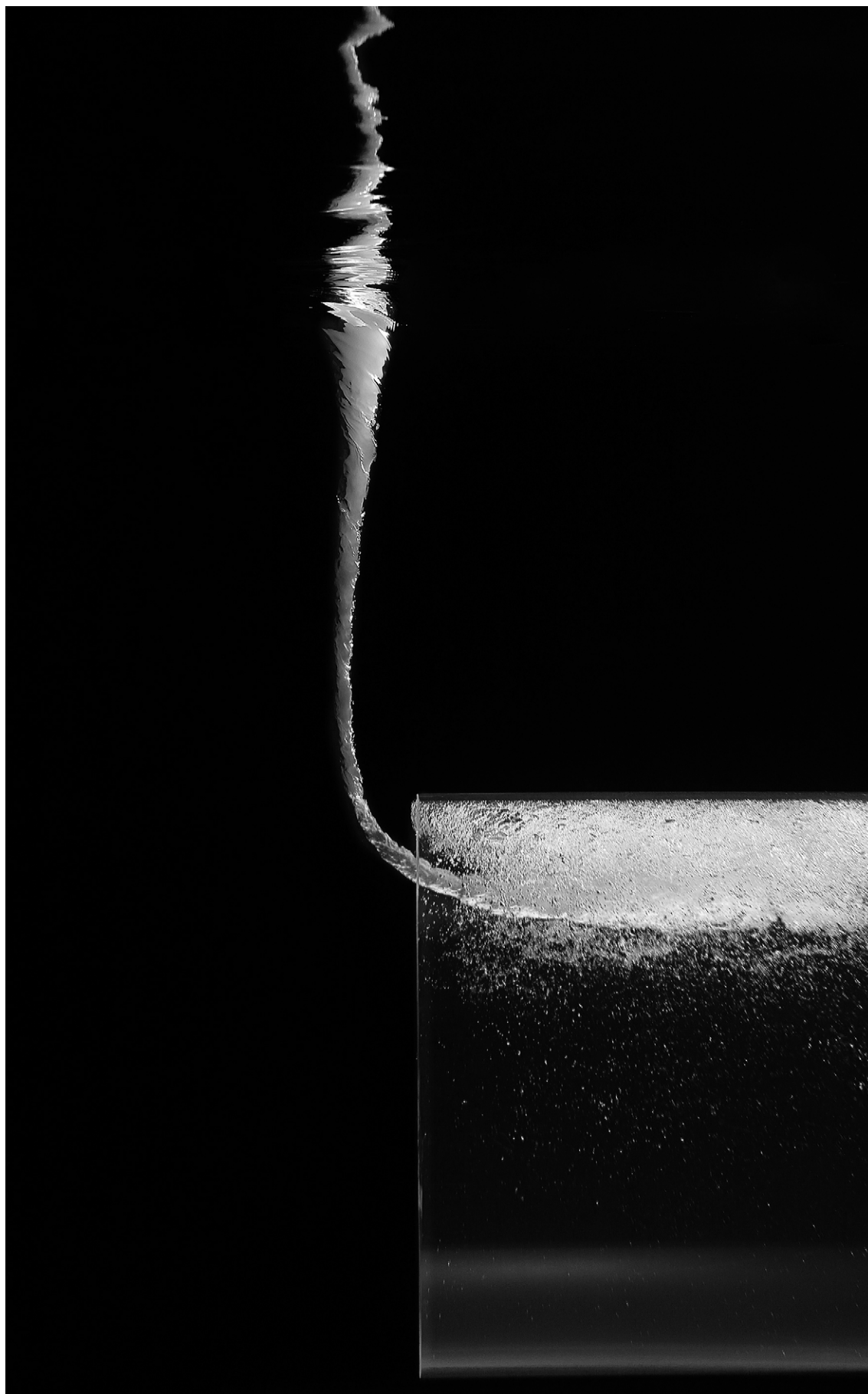
Figure 7.5: Air-core intake vortex tube flow visualization by dry ice fog.
