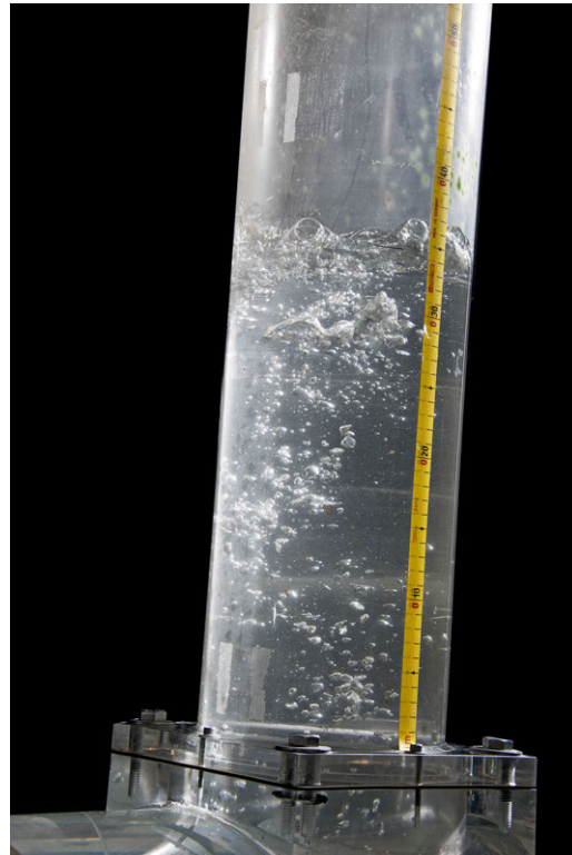
(b) De-aeration at rising pipe #2
