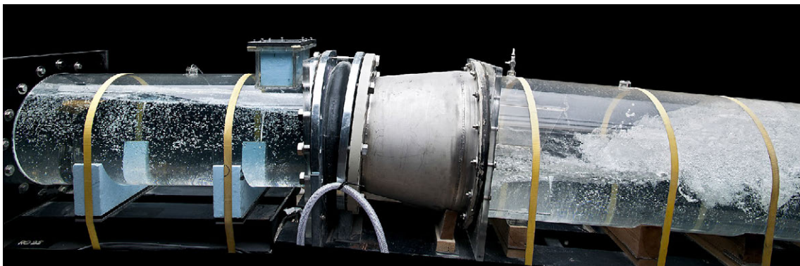
(d) Developed air pocket equals a further developed hydraulic jump, position and size depends on Q_a , t = 200 s
