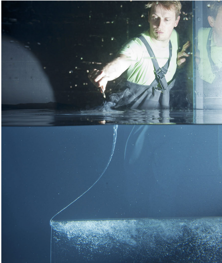
Figure 7.2: Smoke experiment at h/D = 2.0 , F_D = 0.9 to visualize the air flow through the tube of an air-core intake vortex.
