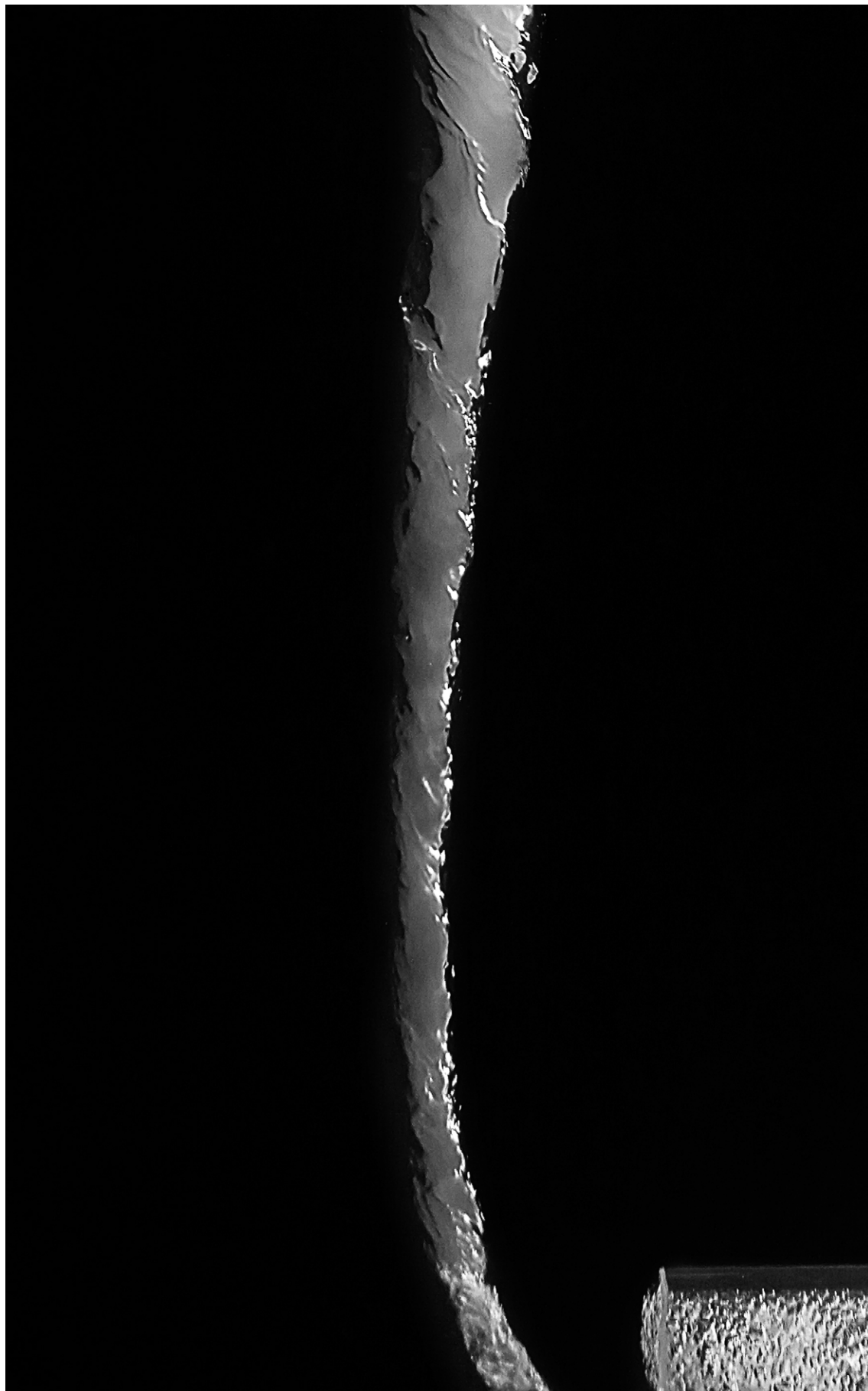
Figure 7.7: Detail (straight air-core) of the air-core tube filled up with dry ice fog.
