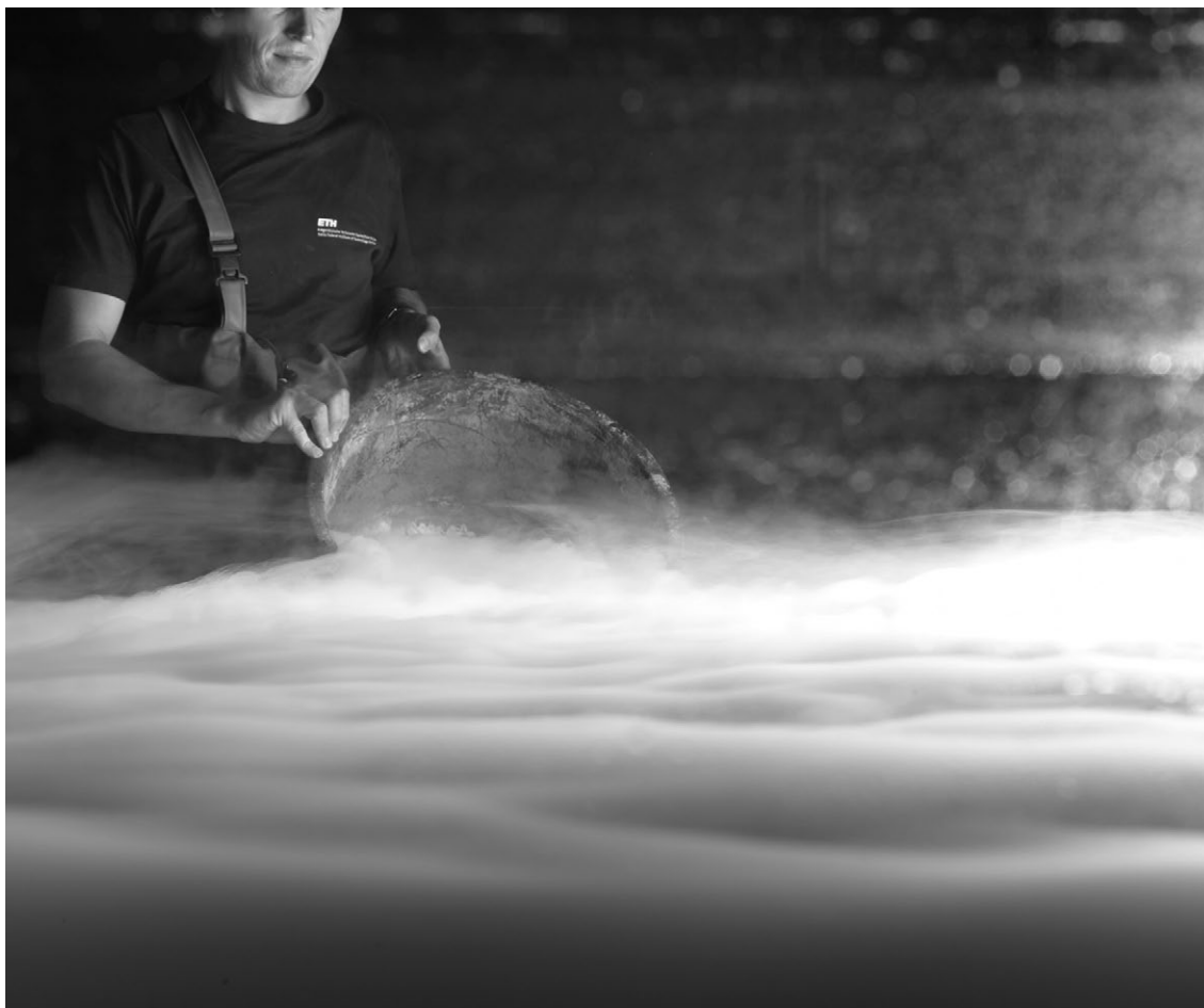
Figure 7.4: Provision of sufficient gas above the water surface by dry ice fog to visualize the flow through the air-core.
