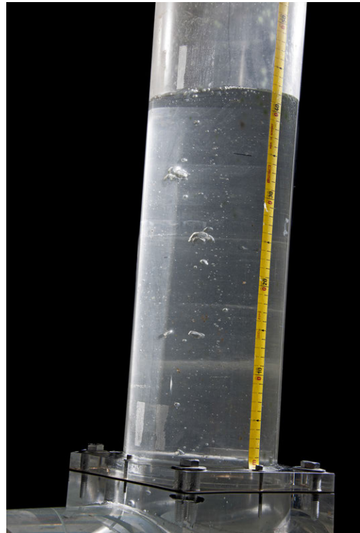
(b) De-aeration at rising pipe #2
