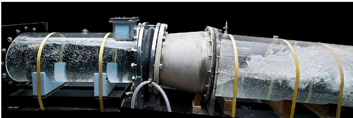
(c) Developed air pocket equals a hydraulic jump, position and size depends on Q_a , t = 180 s
