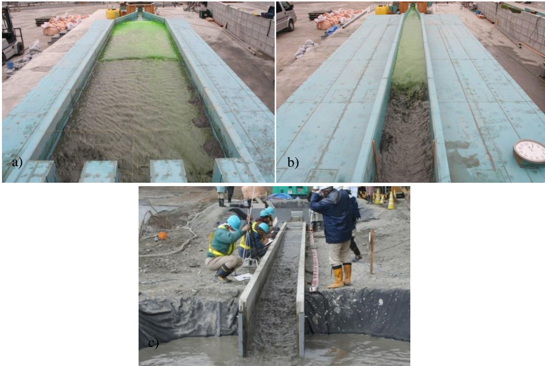
Figure 13: Situation of sediment erosion experiments a) scale 1/25, b) scale 1/15, c) scale 1/5
