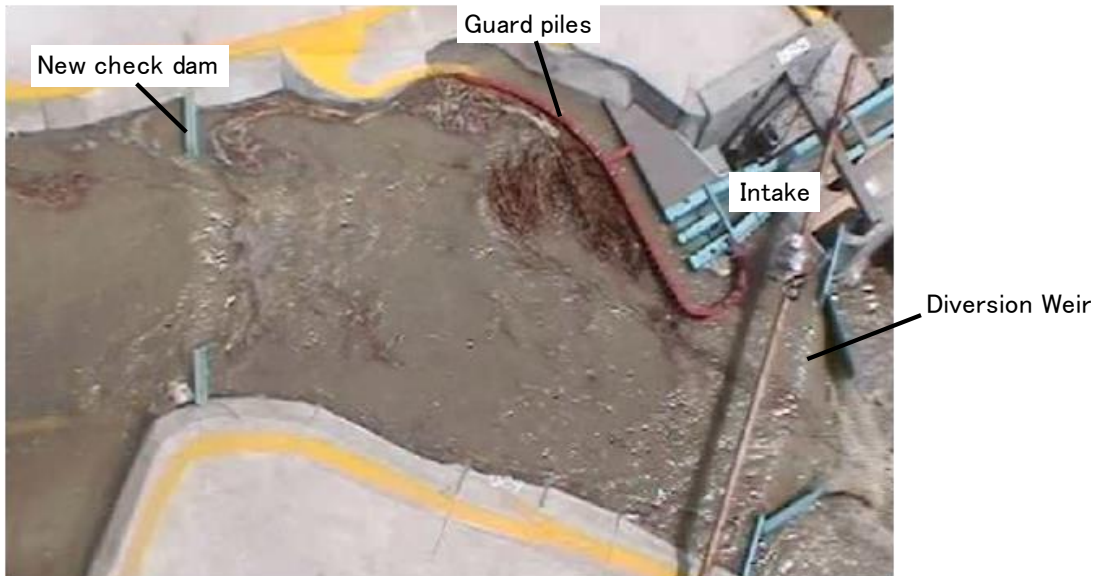
Figure 7: Trapping situation of drift wood ( 1300\text{m}^3/\text{s} )
