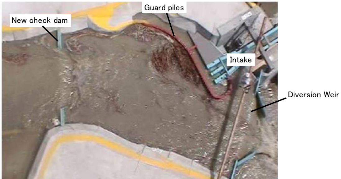
Figure 7: Trapping situation of drift wood ( 1300\text{m}^3/\text{s} )
