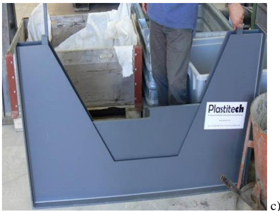
Figure 2: Picture of the physical model constructed at the LCH with its main operational elements (a), the two sill positions (b) as well as the adjustable downstream DS (c) and upstream US sill (d)
