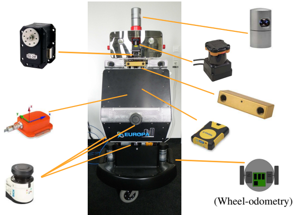
Figure 8.1.: EUROPA2 sensor and actuator setup. The green checks indicate which sensor / actuator is already running and can be calibrated in the EUROPA2 configuration here shown on the ETHZ platform. The question marks indicate sensors or sensor placement, which have not been specified yet.
