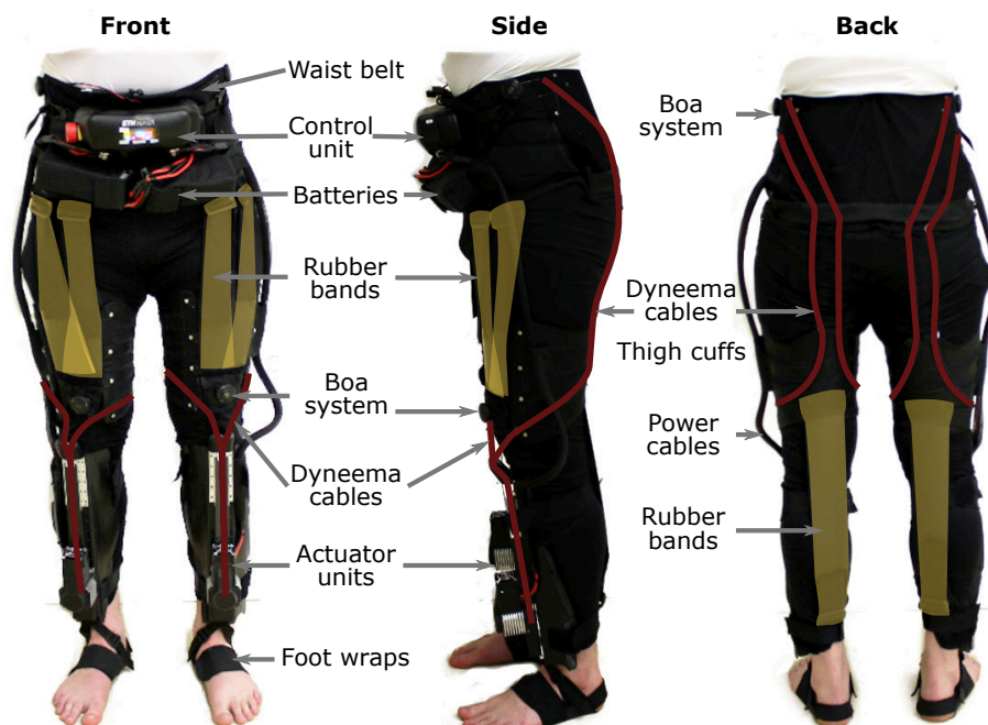
Figure 5.3: System architecture of the Myosuit
