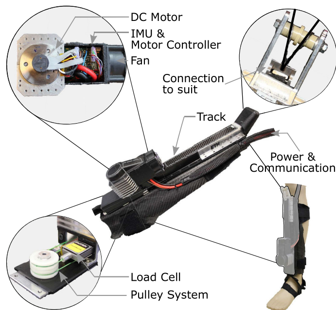
Figure 5.4: Tendon actuator weighing 1070 g.
