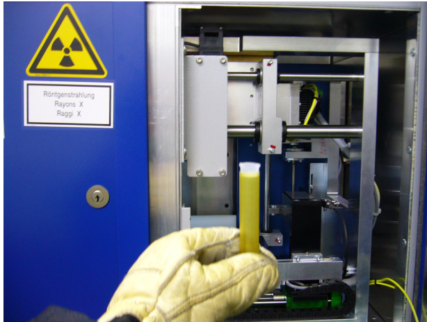
Fig. 2.3: X-ray tomography scanner with a sample holder.
