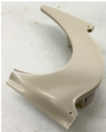
(a) Milled PEEK hub insert
