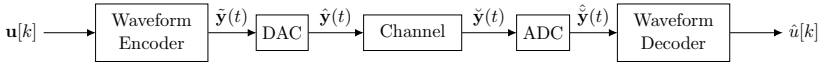
Figure 11.4: A simplified view of a communication scenario describing the steps involved to transmit a digital signal over an analog domain.
