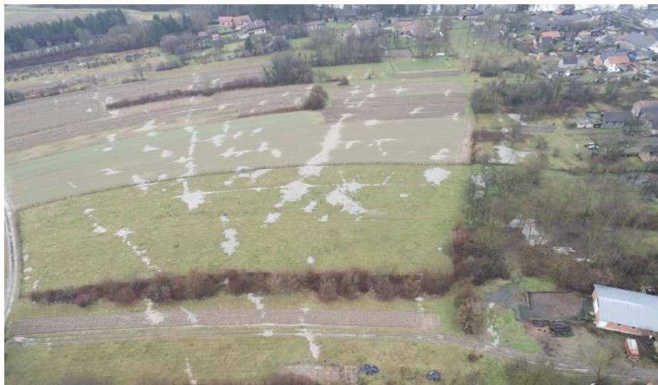
Figure 6.7. Aerial image of liquefaction ejecta at (45°30'41.988"N,16°24'37.632"E, source: Vedran Damjanović).
