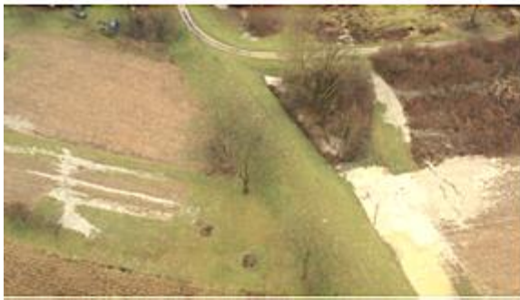
Figure 6.8. Liquefaction near Hrastelnica and Sisak. The proximity of these liquefaction surface manifestations to levees indicates that liquefaction was a definite mechanism contributing to the levee failures (see later subsection). The bottom right image is a close-up of the bottom left (source: Croatian Waters Archive).
