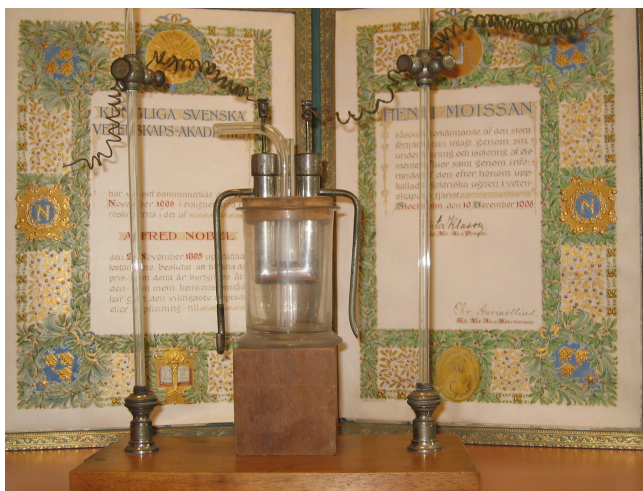
Picture 1: Moissan's apparatus for the isolation of F_2 . From Henri Moissan Museum, Faculty of Pharmacy, University Paris V, Photo Alain Tressaud.
