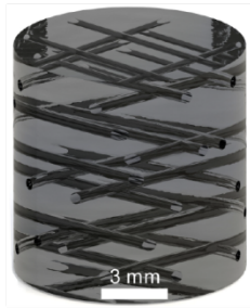
Fig. 1: Sample description. a) 3-D printed samples with no porosity and 5%, 10%, 15% and 20% porosity. b) Schematic illustration of a printed cylinder with 5% pore space. c) Two examples of CT scans for 2-D sections in the X-Z plane for a sample that has not undergone any compaction. It illustrates the preferential alignment of particles in the printing (X-Y) plane.
