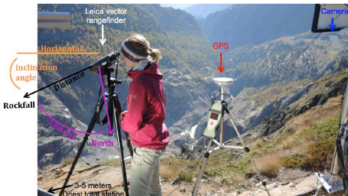
Figure 15: Field installation of the Leica vector and measurement explanation (Photo taken by Andrea Manconi)
