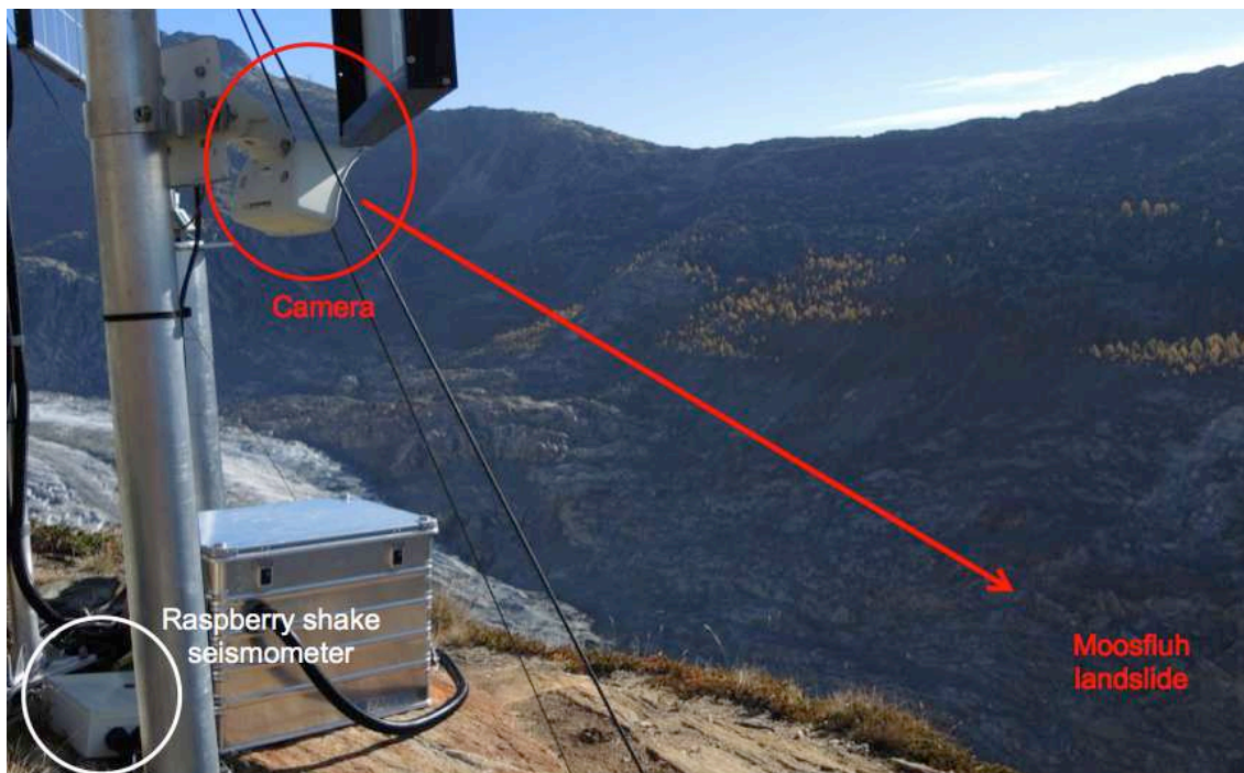
Figure 10: Webcam in Driest oriented towards the landslide, taking photos every 10 minutes to capture the rockfalls
