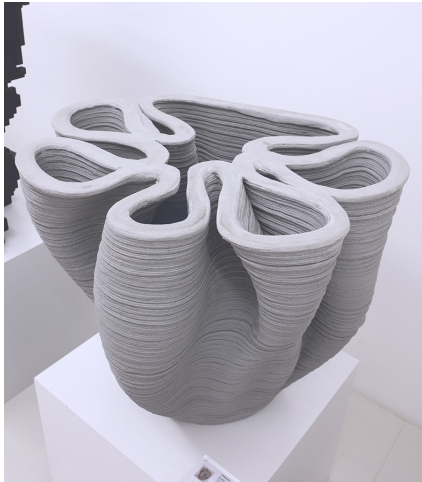
Figure 2.8: Practical implications and challenges of structural build-up control for processing and manufacturing. Achievements in contour length changes in the case of layered extrusion for a piece contracted by Zaha Hadid Architects [99] and of cross-section area for slipforming [42]. Reproduced from [99] and [42].
