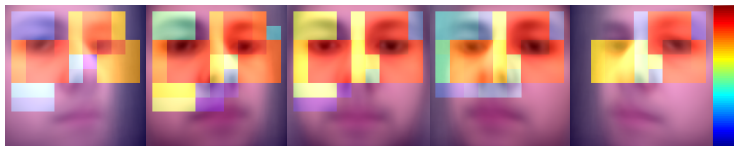
Figure 7: Spatial distributions of selected regions by our three-region model for different horizontal head angles. We visualize the regions' locations using the jet color map and overlay the heat maps on the averaged face images corresponding to each pose.
