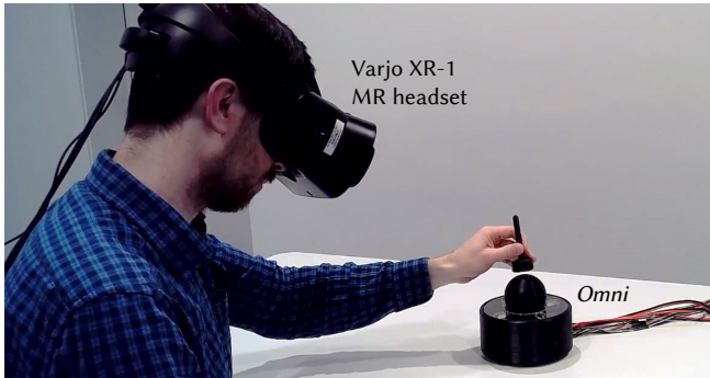
Figure 10. We combine Omni with a video see-through MR device (Varjo XR-1) to showcase the applications.
