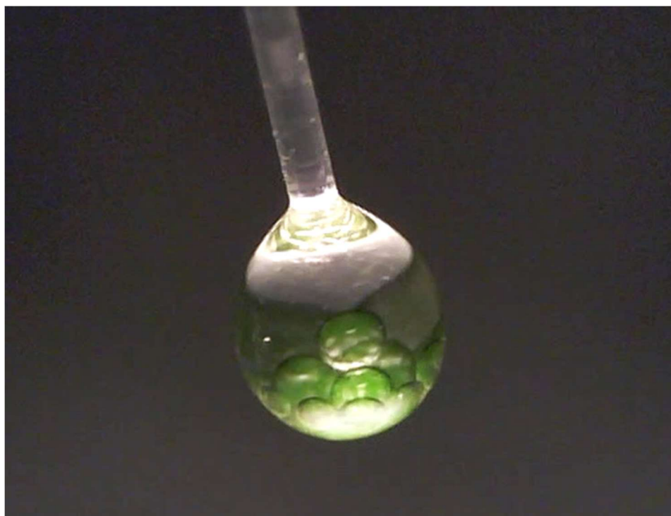
Figure 5-1: Photograph of the spotting capillary with a three-dimensional droplet network in a hanging drop. The aqueous phase consisted of 50 \mu M rhodamine 6G in 20 mM MES and the oil phase consisted of 0.625 mM DOPC in 1:1 hexadecane/squalane.
