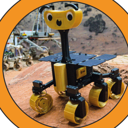
Figure 3. ExoMy uses off-the-shelf components, making it easily reproducible.
