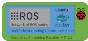
Figure 5. Running ROS in an Ubuntu docker container allows reliable installations.
