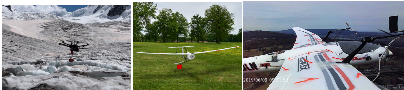
Figure 9.1: Future fixed-wing UAV applications: (Left) Dropping a GNSS station on the Gorner Glacier, Switzerland, from a MAV. (Center) Rendering of fixed-wing payload recovery. (Right) The Easy Glider UAV in stabilized deep stall.
