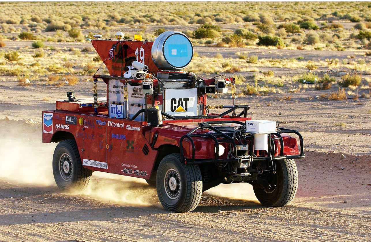
Figure 1.1 Carnegie Mellon's off-road driving robot, Sandstorm Red Team's car that went the furthest in the 2004 DARPA Grand Challenge Source: cs.cmu.edu
