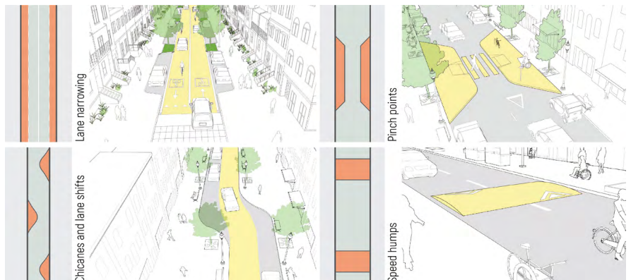
Figure 10.7 Some traffic calming strategies From NACTO's Global Street Design Guide. Source: globaldesigningcities.org
