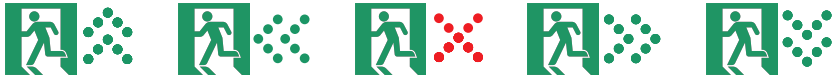
FIGURE 5.2: Evacuation sign design. The four arrow designs were applied and animated with scrolling motion in both the non-adaptive and adaptive sign conditions. The blinking red "X" only appeared in the adaptive sign group.
