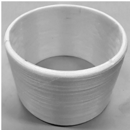
Figure 11.1: _____ Cake of polycarbonate-clad glass monofilament as obtained from the spinning process. Its inner diameter is 135 mm and its height is 80 mm.
