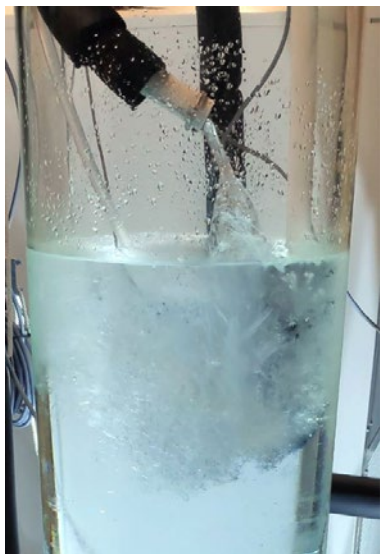
Figure 5: Glass container filled with water and floating ice crystals. Supercooled water flows into the container through a hose (top left) and turns into ice slurry as soon as it hits the floating ice crystals.
