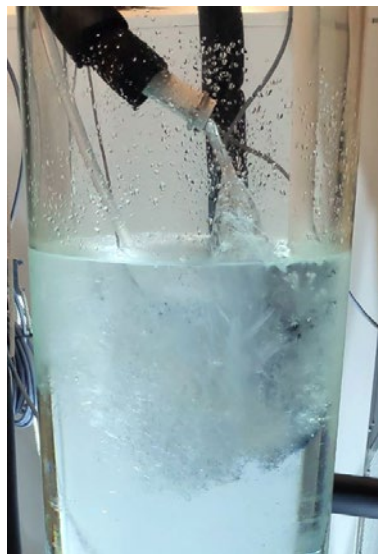
Figure 5: Glass container filled with water and floating ice crystals. Supercooled water flows into the container through a hose (top left) and turns into ice slurry as soon as it hits the floating ice crystals.
