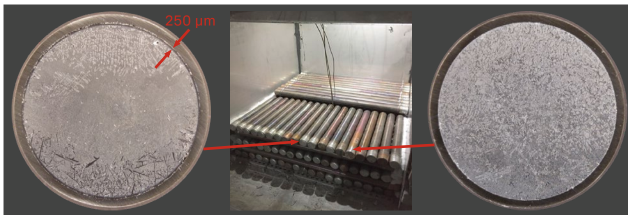
Figure 3: Centre: Latent thermal storage unit partially loaded with steel tubes. When completely loaded, the unit contains 296 steel tubes each filled with an aluminium-copper-silica alloy. Left: Cross section through a tube without a diffusion barrier. After exposure to high temperatures for about 100 hours, a 250 \mu\text{m} thick intermetallic layer has formed. Right: Cross section through a tube with a diffusion barrier; despite the high temperatures, no intermetallic layer has formed.
