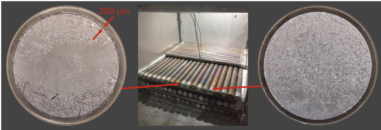
Figure 3: Centre: Latent thermal storage unit partially loaded with steel tubes. When completely loaded, the unit contains 296 steel tubes each filled with an aluminium-copper-silica alloy. Left: Cross section through a tube without a diffusion barrier. After exposure to high temperatures for about 100 hours, a 250 µm thick intermetallic layer has formed. Right: Cross section through a tube with a diffusion barrier; despite the high temperatures, no intermetallic layer has formed.
