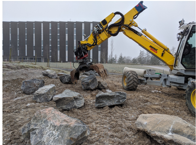
Fig. 3 Initial state of stones, loosely distributed on the terrain. LiDAR mapping and RANSAC ground segmentation allows for initial detection and grasping for refined scanning in the gripper.
