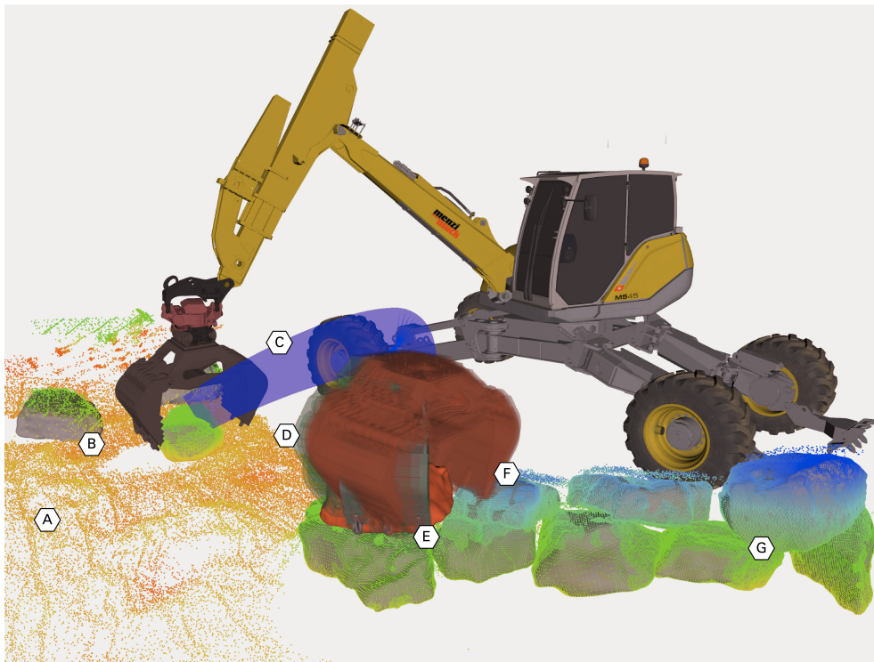
Fig. 7 Grasp planning and placement of a stone to its desired location (red). (A) Collision and localization point cloud, (B) Stones localized in point cloud, (C) Spline motion trajectory, (D, Green) Collision free grasp hypotheses, (F, Red) Grasp hypotheses with collisions, (E) Selected grasp configuration, (G) The collision point cloud is augmented with point clouds of already localized stones.
