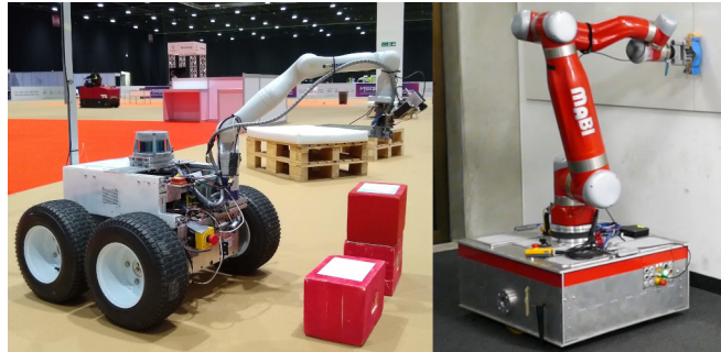
Fig. 1: Two mobile robots performing manipulation tasks. Left: Swaco picking up a brick for the MBZIRC2020 robotics competition. Right: MabiMobile cleaning a whiteboard by controlling the interaction force.
