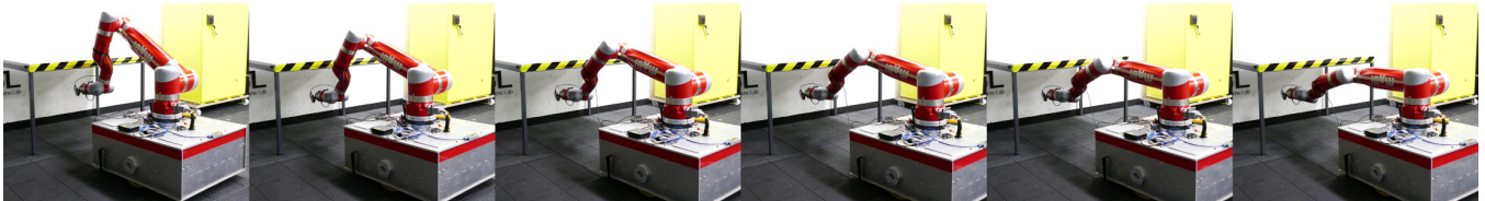
Fig. 3: Collision avoidance hardware experiment: The robot reaches underneath the table. The base first moves back such that the arm does not collide with the top of the table.
