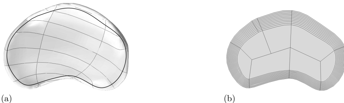
Figure 9.6: Topview on spline based model imported from GEOMAGIC into ABAQUS with superimposed approximate contour (a). This contour is used to create a template geometry with NP and ten AF layers (b).
