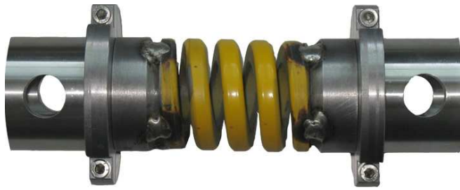
(a) steel spring welded to steel adapters
