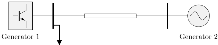
FIGURE 4.2: Configuration of the investigated system comprising two generators and one load connected via a transmission line.
