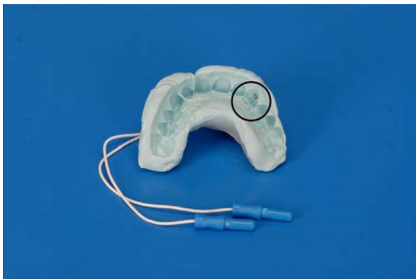
Figure 3. Exemplary dental splint for electrical dental stimulation. The electrical stimulus is applied via the embedded electrodes located at the palatal and labial surface of the right upper canine indicated by the black circle.
